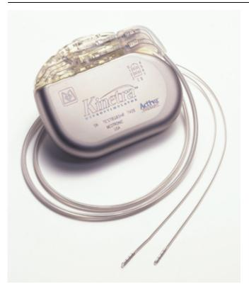
The Kinetra neurostimulator works through 2 channels to deliver bilateral therapy with a single device.
